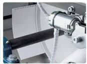
Turnover drum keeps the punched sheets in the correct page sequence and delivers them to the ejection system. Handling paperweights from 60 up to 800 gram.
