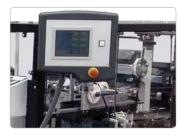
Touch screen setup with up to a 50 job memory capacity.
